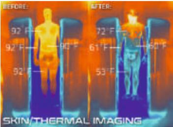
Thermovision camera (thermal+ lat. visio "vision") is a device for monitoring the temperature distribution of the examined surface. The temperature distribution is shown on the display as a color picture, where different temperatures correspond to different colors. The study of thermal images is called thermography. All bodies whose temperature exceeds the temperature of
